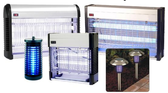
Our electronic high efficiency flying insect killer machines attract the insects and kill them instantly with a mild electric shock. Insect killer and fly catcher machines work on the principle of luring mosquitoes and flies towards the specialized tube lights installed in the system and once the insects touch the high voltage wires surrounding the tube light the instantly get electrocuted.
